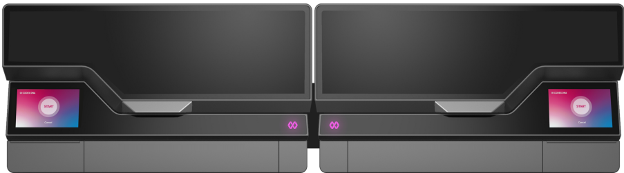
Figure 11: Our BioXp DBC system for fully-integrated on-demand writing of synthetic DNA, mRNA and protein
